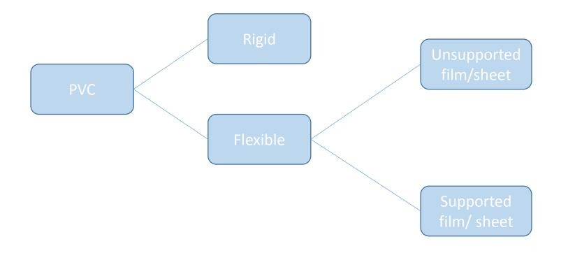
A variety of fPVC manufacturing technologies exist. Calendar and blown films are typically used to create unsupported PVC whereas knife over roll, lamination and extrusion are often utilized to create supported flexible PVC products.
